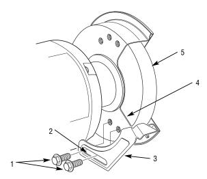
FIGURE 2. INSTALLING THE R/H TOOL REST
